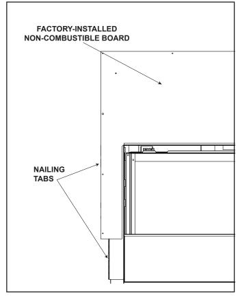
Figure 13.1 Nailing Tabs Installation Position
